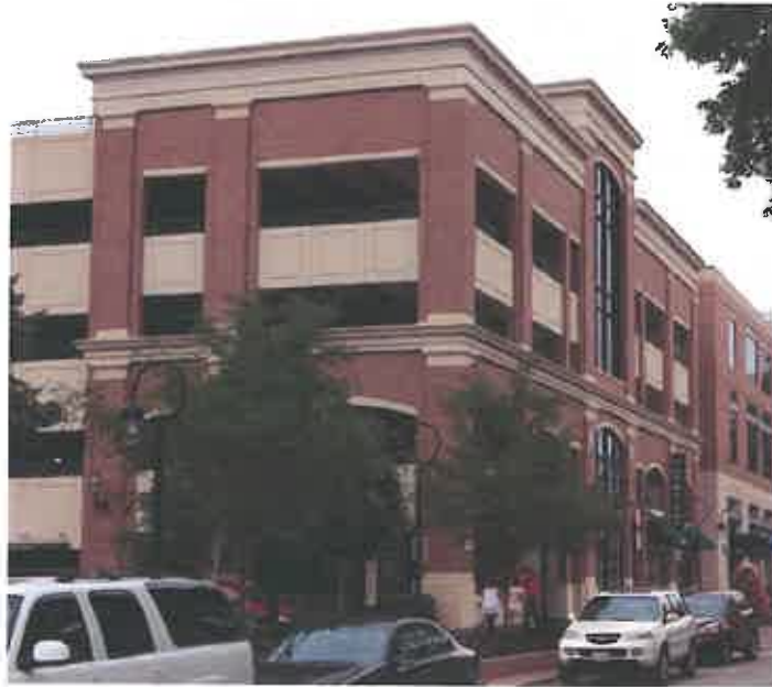
Figure C2.1a: Vertical brick articulation combines with horizontal stone/ precast concrete banding to form overall grid frameworks. Cornices unify the top of the building.
