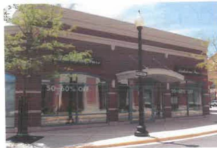
Figure B4.4b: Acceptable use of metal awnings
