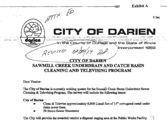
The City will provide the awarded vendor a disposal staging area at the Public Works Facility located at 1041 South Frontage Road. The vendor will be required to utilize a jetter or equivalent, to remove all debris from the existing 15-inch metal underdrain. The catch basins, inlets, and storm manholes, referred to as Storm Sewer Structures shall be cleaned of all debris. The catch basins shall be limited to a cleaning of 2-foot below the existing pipe invert.
