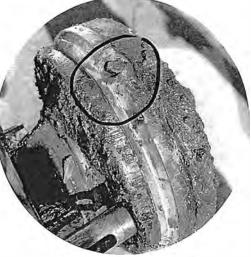
Leak on Corroded Hydrant Shoe
