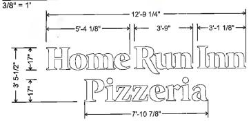
5"deep fabricated face-lit channel letters .040 std. black coil returns with cinched .063 aluminum backs 3/16"thick translucent white polycarbonate faces with 1" std. black trimcap
