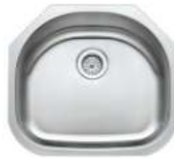
SIN-18-SINBWL-2321 Outside - 23 3 / 4 " x 21" Inside - 21 1 / 4 " x 19" Depth - 8" Minimum Cabinet - 27"
