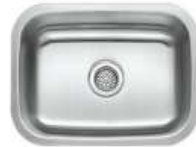
SIN-18-SINBWL-2318 Outside - 23 3 / 16 " x 17 3 / 4 " Inside - 21 1 / 16 " x 15 1 / 4 " Depth - 8" Minimum Cabinet - 27"
