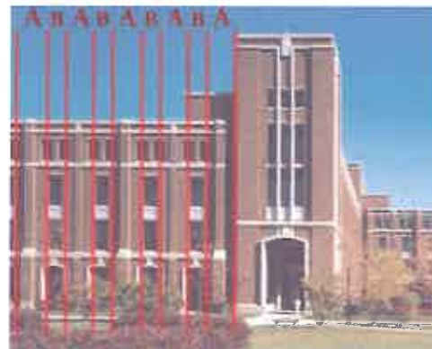
Figure C3.3: Syncopation of façade elements
