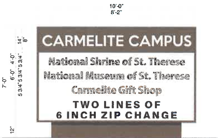
SIGN #1 ONE (1) D.F. LED ILLUM. MONUMENT DISPLAY 3/8" = 1'-0" SIGN TO BE DURANODIC BRONZE. WHITE LEXAN FACES W/ 3M 230-69 DURANODIC VINYL COPY.
