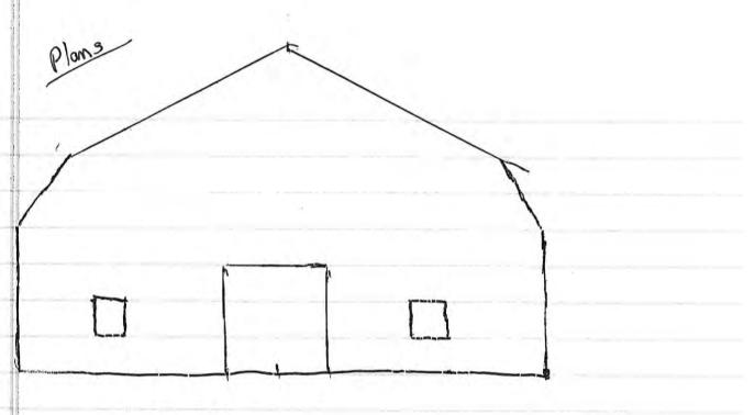
2X4 16" O.C. 2X8 FRAME FOR DECK 1/2" PLYWOOD FOR WALLS & ROOF 3/4" PLYWOOD FOR DECK
