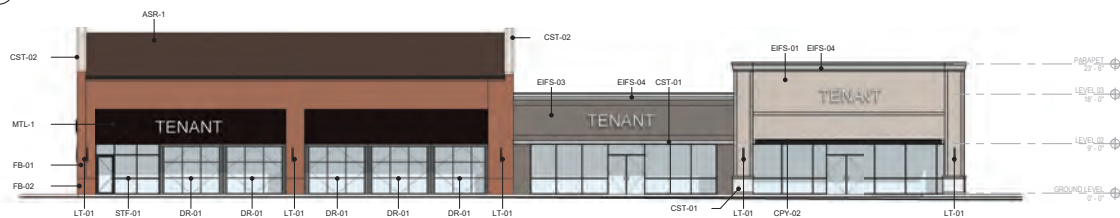
2 NEW WEST ELEVATION - RETAIL F SCALE: 3/32" = 1' 0"
