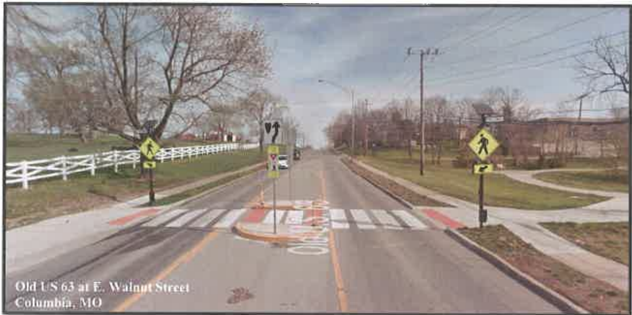
Figure 12 Example of Recommended Midblock Pedestrian Crossing Treatment
